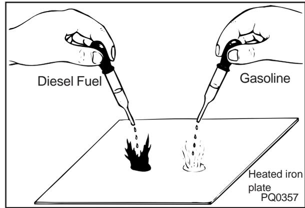
In a diesel engine, in which fuel is burned by the compressive heat of the air, ignitability is an important characteristic. It greatly influences the length of time after the fuel is injected into the combustion chamber until it starts to burn, which is called the “ignition lag time”.
