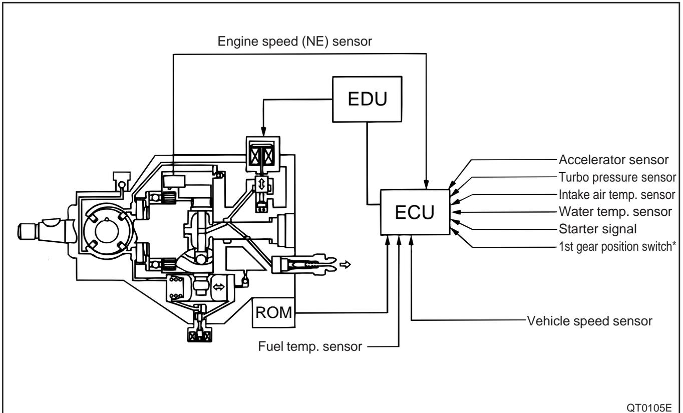
\* : With an M/T vehicle, the 1st gear switch activates the power control to protect the drive system during high load operation.
