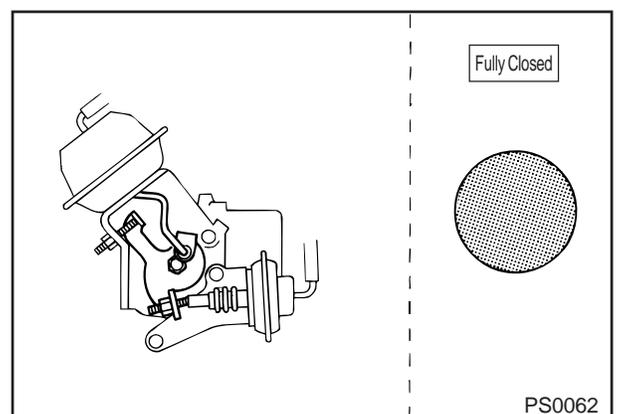
**[Reference: Singel-Valve Type Venturi Intake Air Restriction ontrrol (Example: Electronically Controlled Type Venturi [made by another company])**
