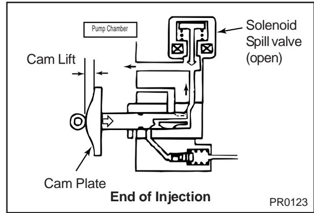
The diagram on the right shows the relationship between the timing in which the cam lift and the solenoid spill valve open and the injection volume.
