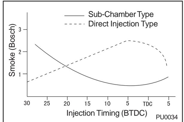
c. Generally speaking, the optimal injection timing for favorable black smoke conditions is later than the optimal injection timing for favorable fuel conditions.
