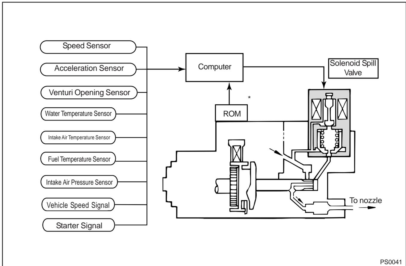
\*Or, correction resistors ( $\theta$  resistors) on conventional type
