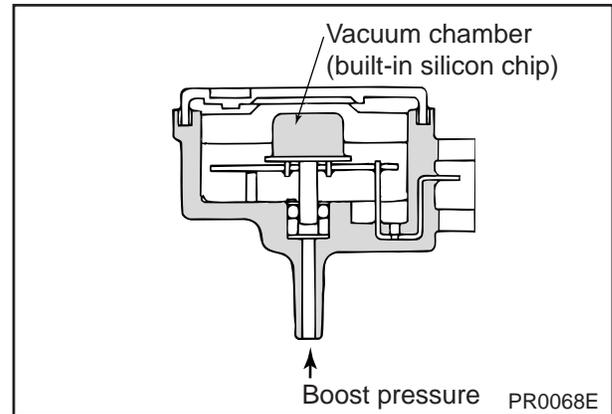
A crystal (silicon) is sealed inside the sensor. This crystal has the characteristic of changing its electric resistance when pressure is applied to it. The turbo pressure sensor is a type of semi-conductor pressure sensor that utilizes this characteristic.
