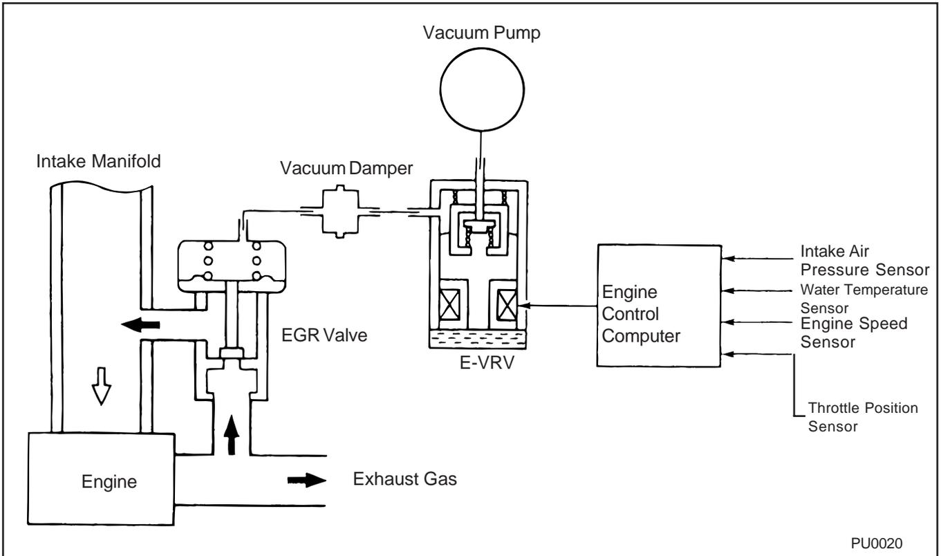
Based on the acceleration opening (throttle position sensor), engine speed, coolant water temperature, intake air pressure, and intake air temperature signals, the computer determines the volume of the recirculation of the exhaust gases and effects duty-cycle control in the operation of the vacuum control valve (E-VRV).
